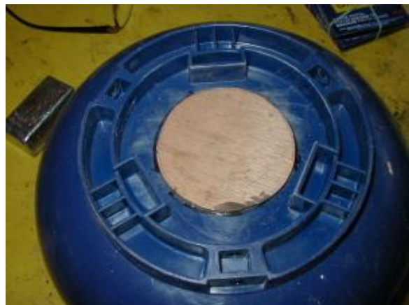
Wooden disk epoxied on cracked bottom
