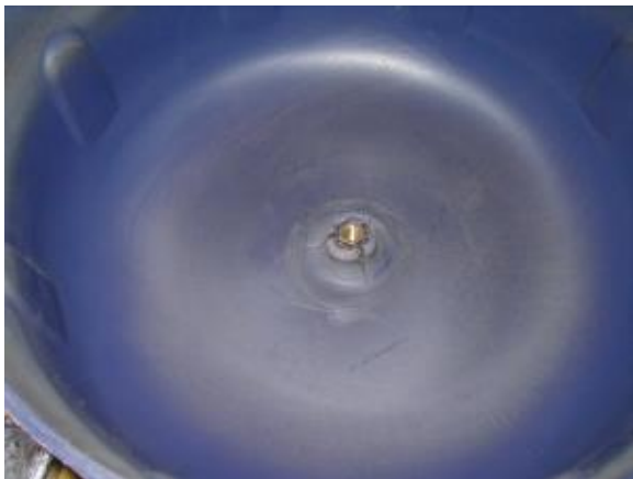
Bowl cracked around nut
