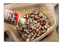
Another low-tech method is to coat the entire bullet with a thin lube solution and let it dry before handling the bullets. Lee Alox is probably the best known of these. The only cost is the Alox and some gun shops actually give bottles of this away. While not as messy as finger-
