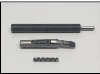
From top: punch, extractor, extra spring
